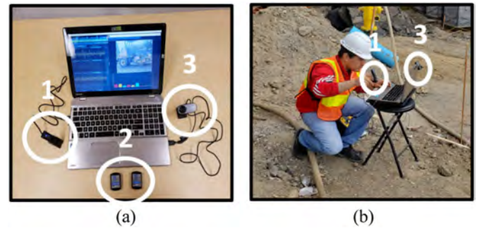
Fig. 1. (a) The Noraxon sensor set: 1. Radio antenna 2. MyoMotion sensors 3. Logitech C270 webcam and (b) Data collection underway at an actual jobsite.
